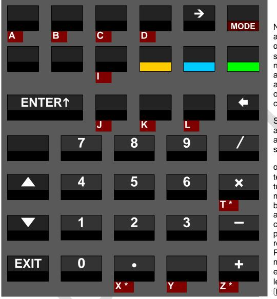
Note all keys are primary in  $\alpha_T$  mode – no shift keys are needed. This allows for fast and easy input of a limited character set.
