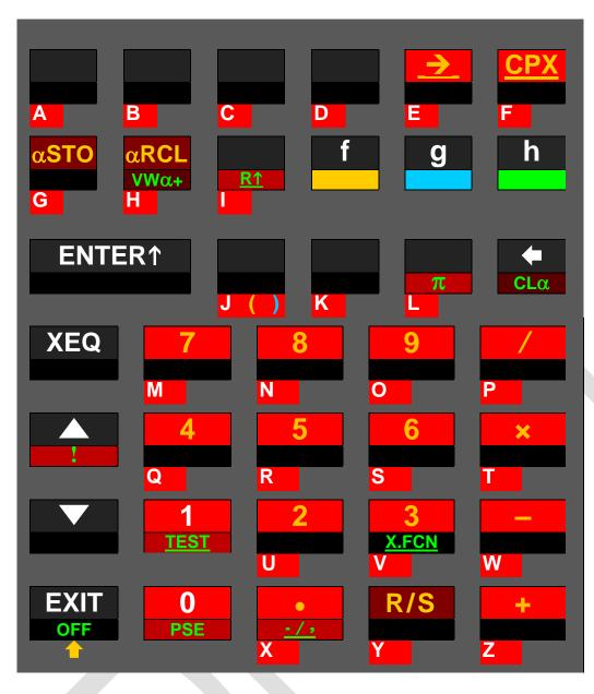
All labels printed on red background in this figure append corresponding characters alpha directly or via alpha catalogs. Note there are some catalogs at new locations in this mode.
