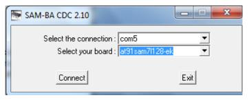
Choose the correct connection (take the port you put your cable in – it may differ from what is printed here). Select the board built in your calculator (i.e. AT91SAM7L128-EK as shown). Press [Connect] then. This was step 6.
