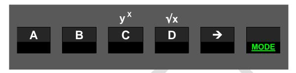
In <u>hexadecimal</u> integer mode (i.e. base 16), on the other hand, primary functions of these top keys will be reassigned automatically, becoming direct numeric input:
