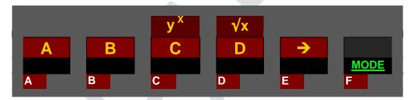
The dark red background is used to indicate changed key functionality in this figure – and this holds for following figures of this kind as well. White print will denote primary functions always (e.g. the top right key enters the digit F in hexadecimal mode immediately). What is printed white on the physical device, is called a <u>default</u> primary function. Wherever such a function is not primary anymore after reassignment, prefix will allow for accessing it (e.g. D will call x here 5).
