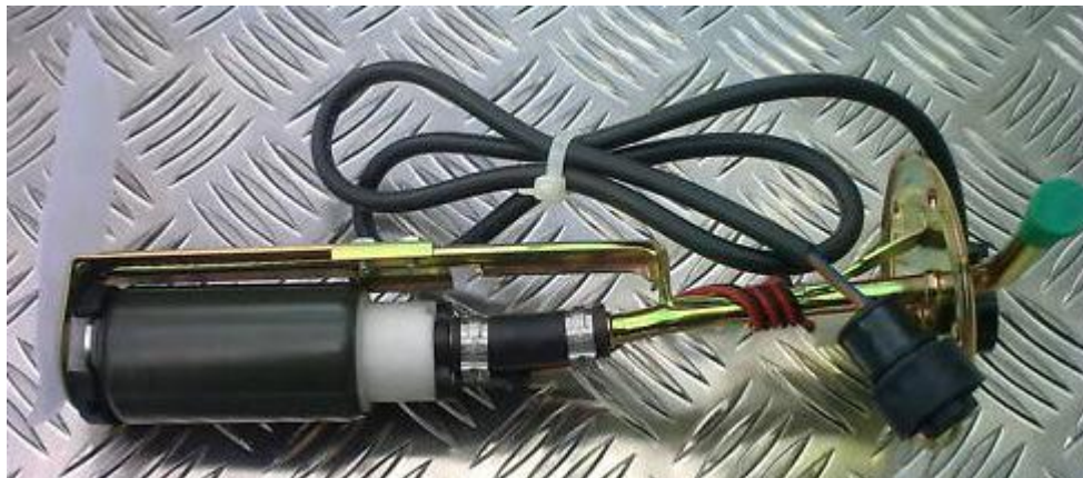
Figure 37 – Web pump for range rover classic (part number PRC 8318)
