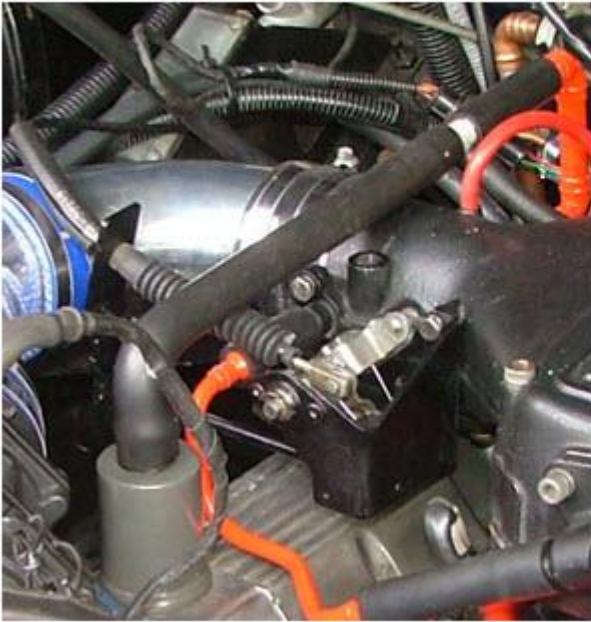
Figure 33 – View of the PCV system pipe routing
