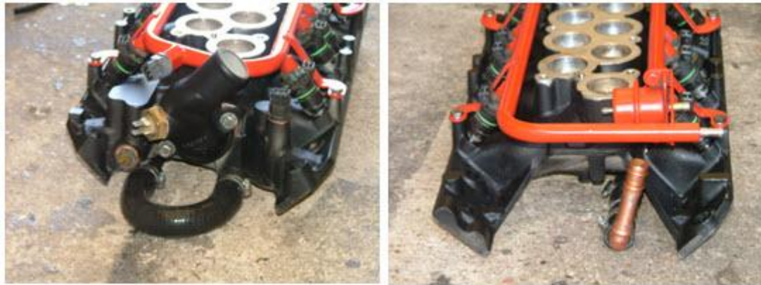
Figure 18 – Intake front and rear view
