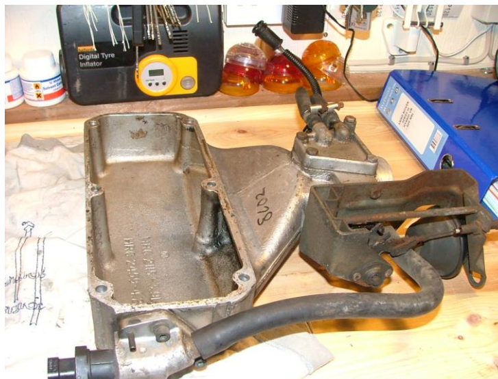
Figure 6 – Underside of plenum.
