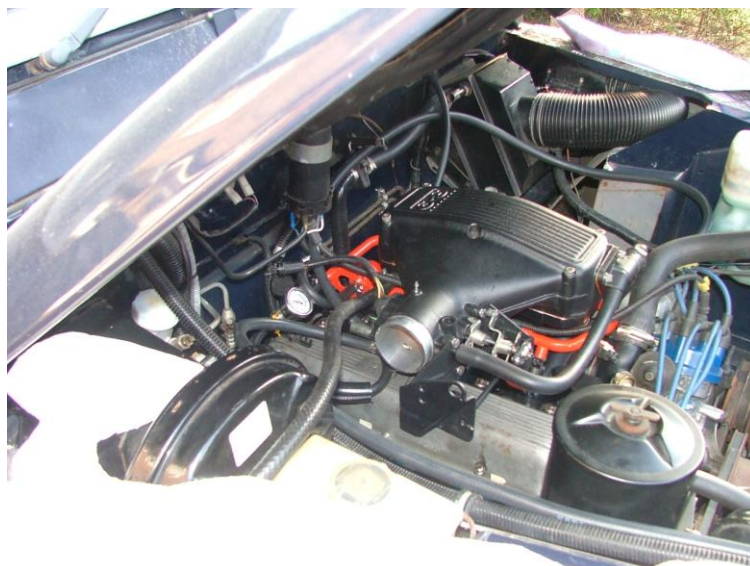
Figure 22 – Final position of the plenum
