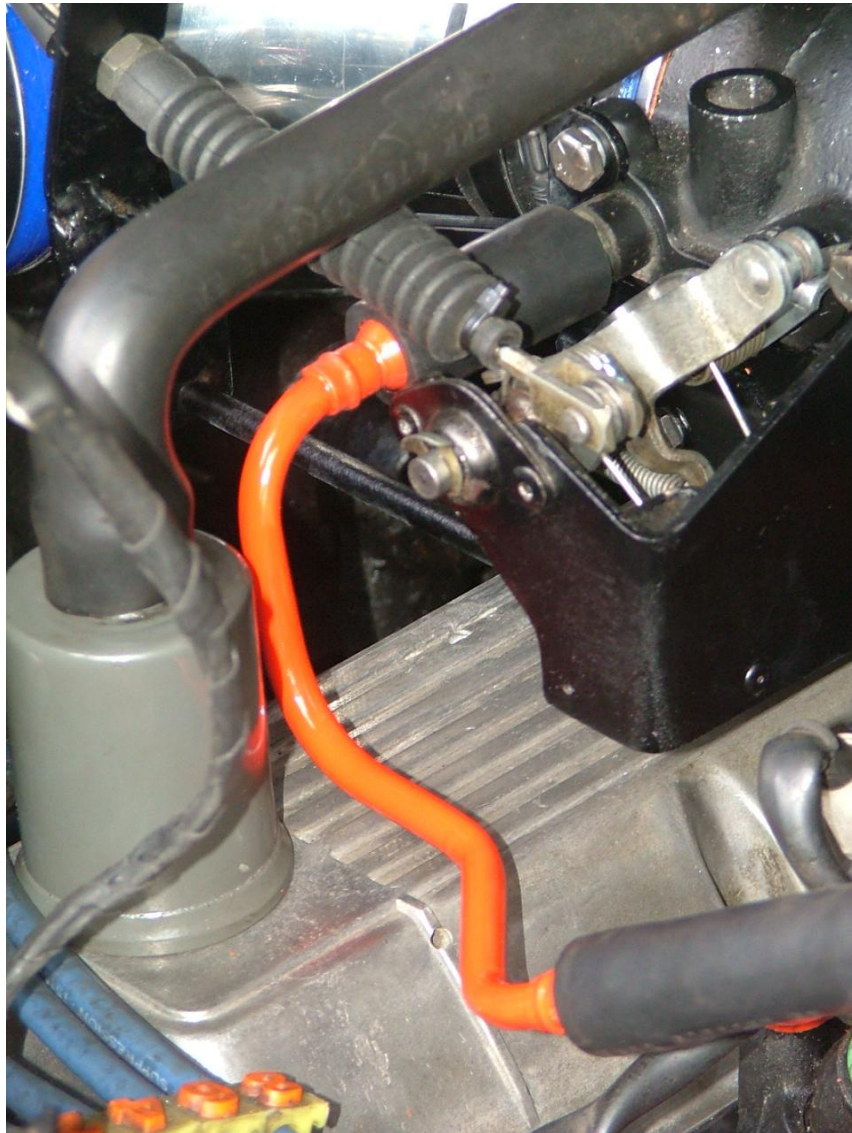
Figure 50 – Idle air supply pipe (red) – no longer used
