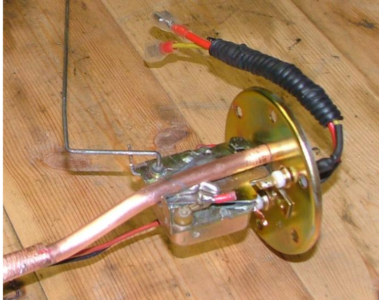
Figure 46 – Electrical module fixed onto the back plate
