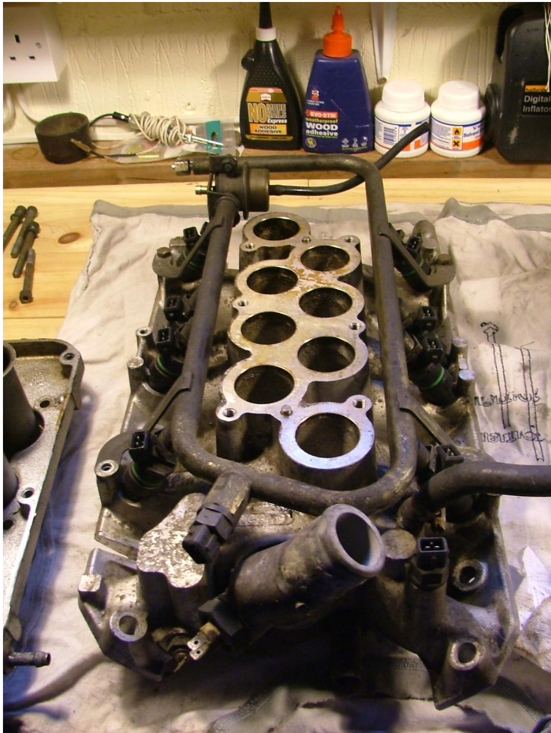
Figure 4 – View of stripped intake manifold
