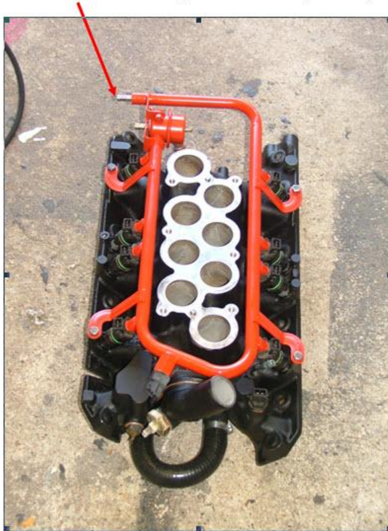
Figure 20 – Finalised injection intake base
