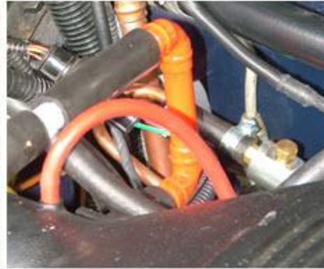
Figure 33 – View of the PCV system pipe routing
