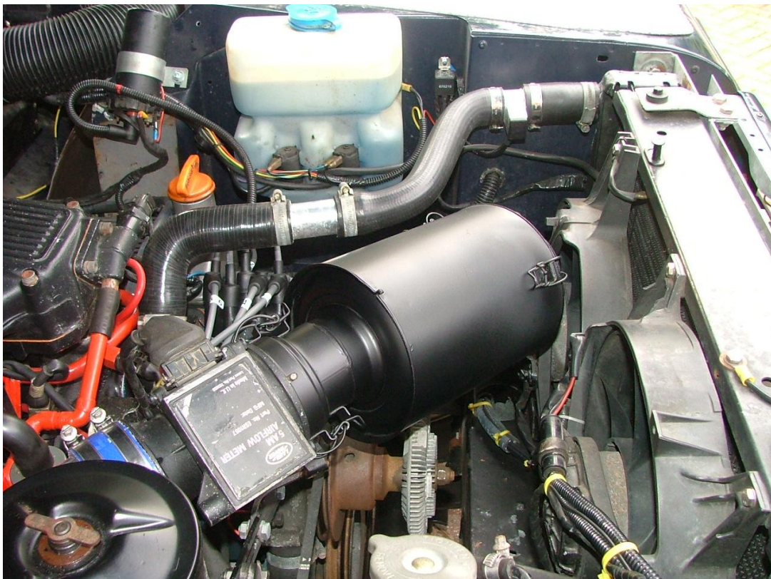
Figure 30 – Modified air cleaner box rear view (note MAF sensor clips)
