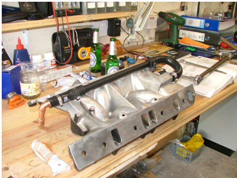
Figure 16 – Underside of injection manifold
