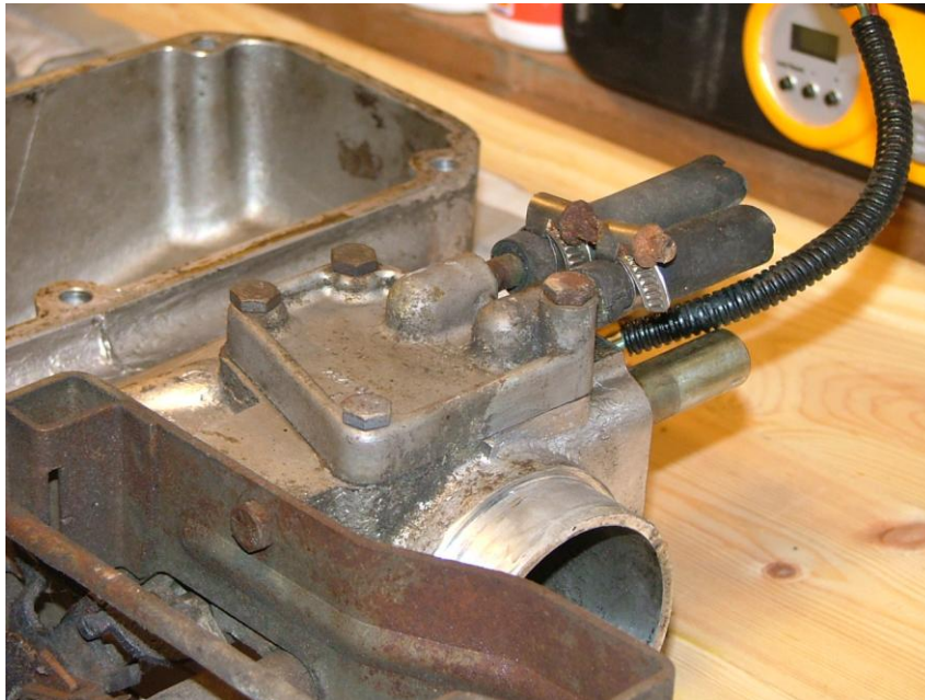
Figure 7 – Close up of plenum chamber pre-heater
