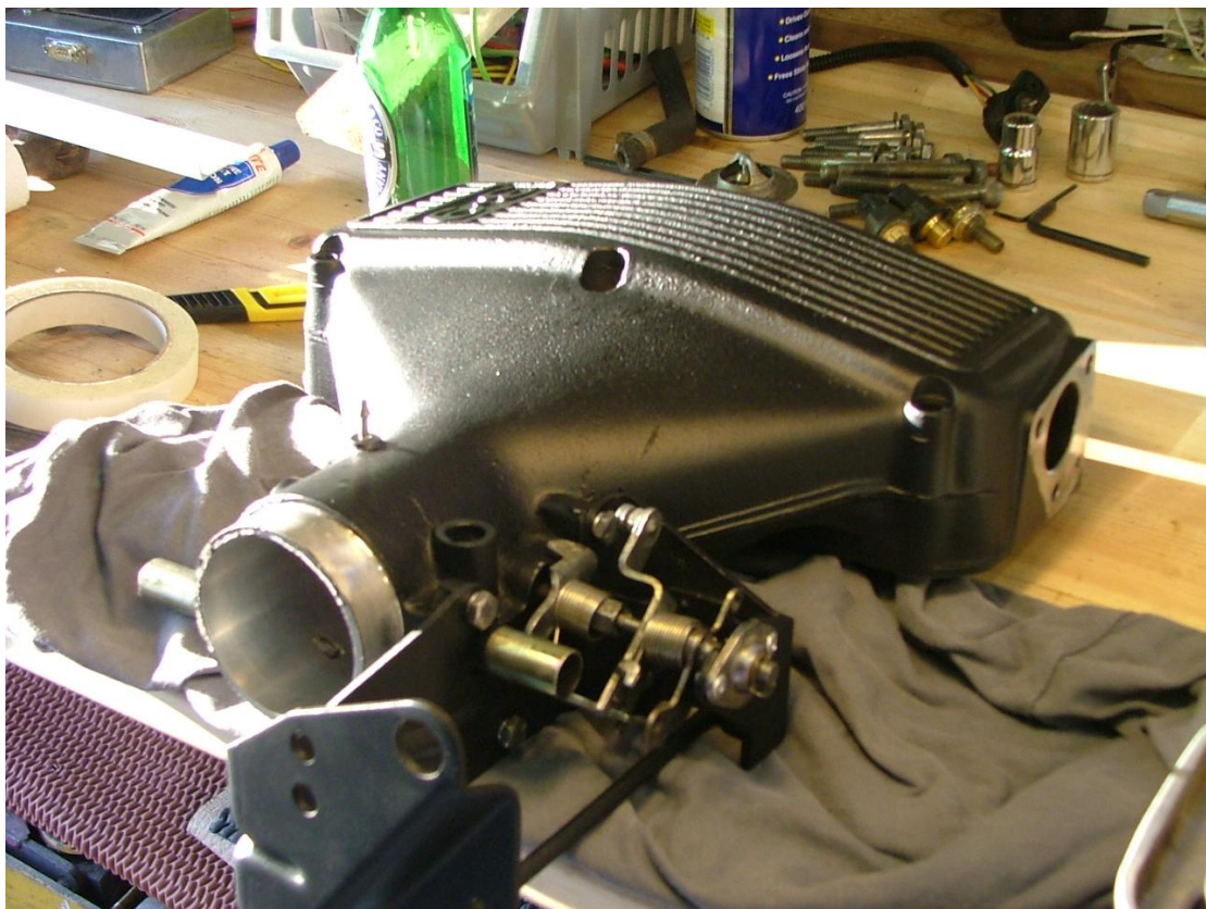
Figure 12 – Sprayed plenum complete with rebuilt throttle linkages
