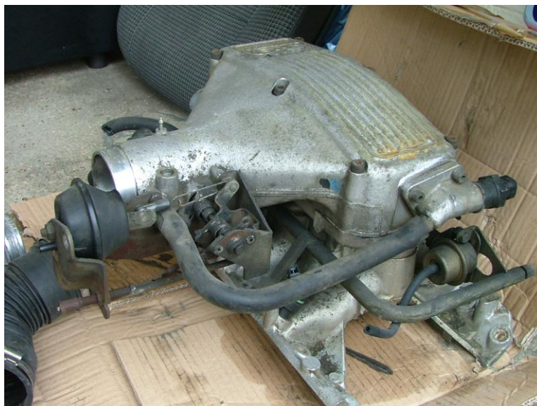
Figure 2 – Plenum side view
