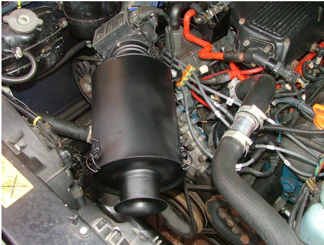
Figure 29 – Modified air cleaner box used to weather proof the intake air filter
