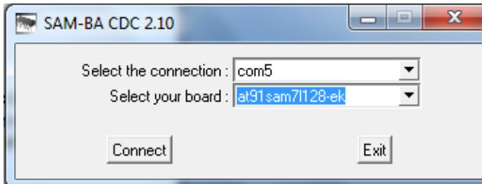
Choose the correct connection (take the port you put your cable in – it may differ from what is printed here). Select the board built in your calculator (i.e. AT91SAM7L128-EK as shown). Press [Connect] then. This was step 6.
