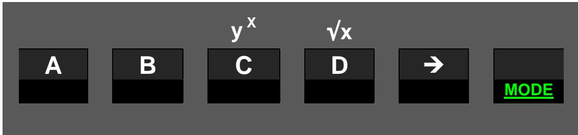
In hexadecimal integer mode (i.e. base 16), on the other hand, primary functions of these top keys will be reassigned automatically, becoming direct numeric input:
