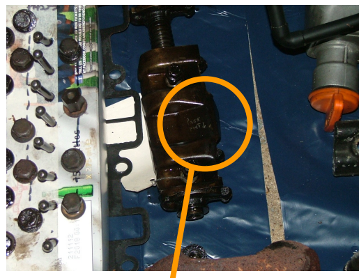
Splash shield marked PASS-FNT ↓ The arrow points to the front of the engine
