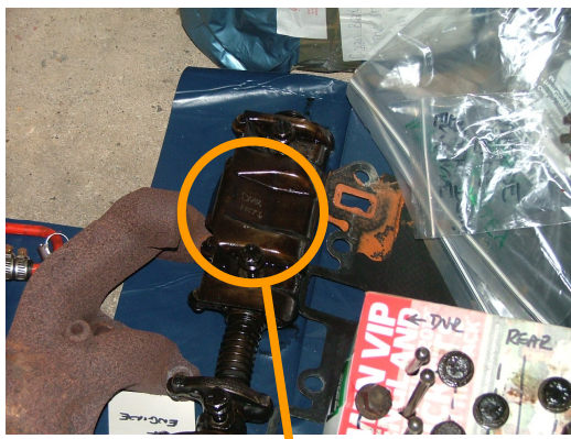
Splash shield marked DVR-FNT ↓ The arrow points to the front of the engine
