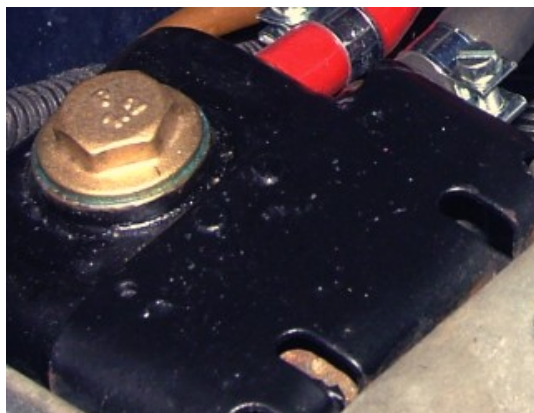
Figure 19 – ½" BSP plug bolt on radiator
