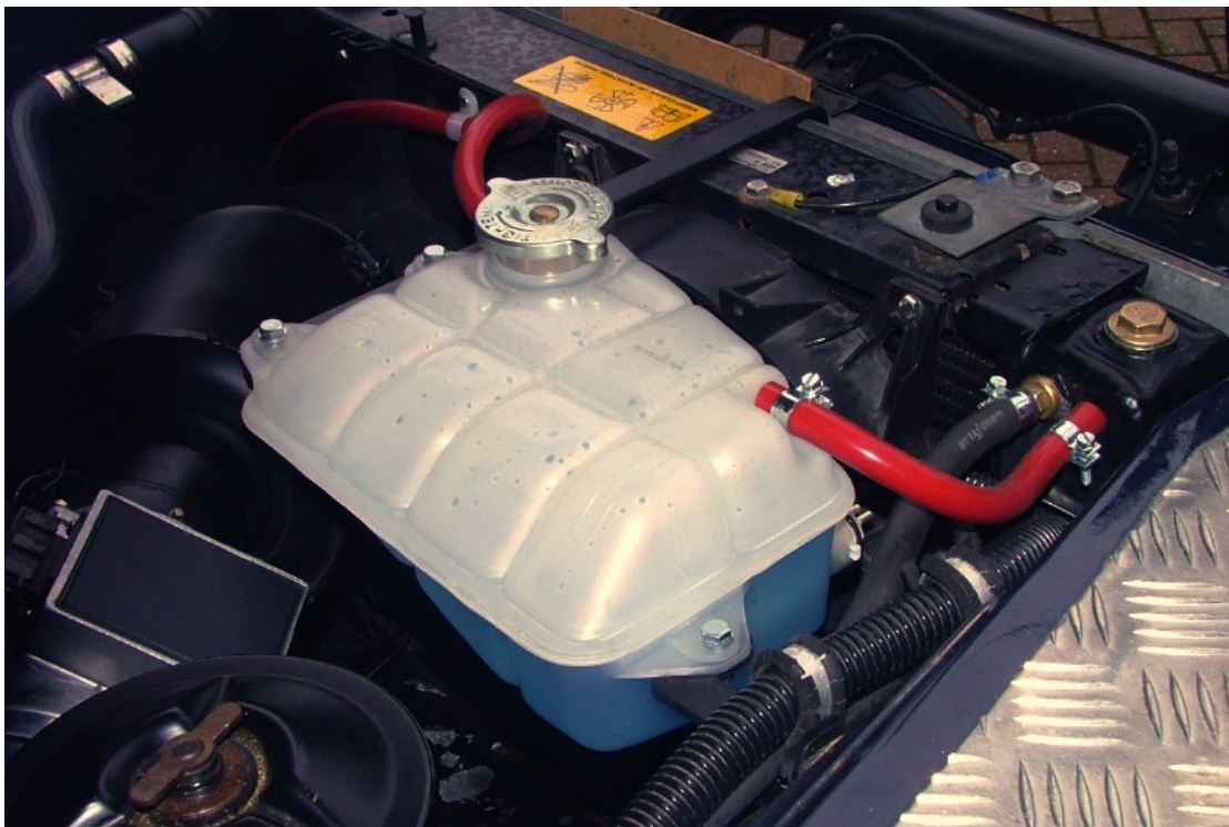
Figure 23 – Final fixing viewed from drivers side rear
